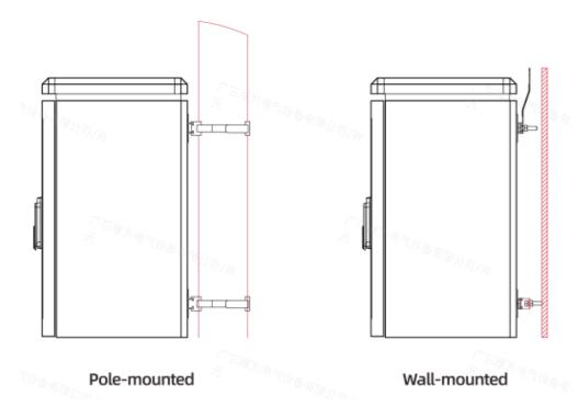
Different installation parts can be purchased for pole, wall or floor installation.
