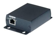
800916 is a POE repeater to extend power and data an additional 100meters. Multiple units are allowed for longer distance, eliminating the need for additional switches, hubs and expensive fiber installations. It compliant with standard POE IEEE802.3af.
