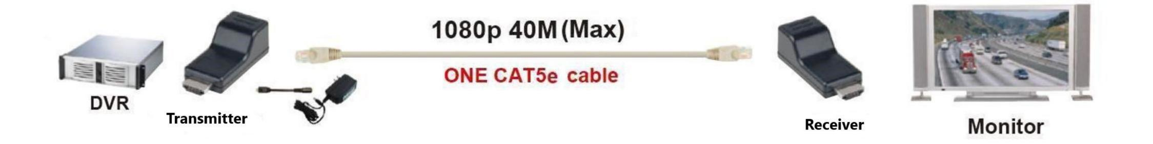
800359 transmitter built in micro USB for external power when your HDMI source not able to provide enough power to the receiver. Please use micro USB to DC plug cable with 5V power adaptor (optional order) for external power.
