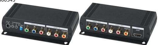
800343 Component Video to HDMI Format converter allow to convert Component Analog Video (YPbPr) + Analog Audio/Digital Audio to HDMI. This converter allows older analog devices to be integrated seamlessly into the modern home theater. It also takes analog stereo audio/digital audio and encodes it onto the HDMI signal for the full HDMI video and audio effect.
